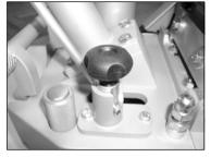
Using the control wheel, the drum pressure can be regulated at high, medium and low in accordance with the following:
