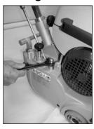
When correctly set, the sanding drum grinds equally across the drum width. If this is not the case, then do the following:
